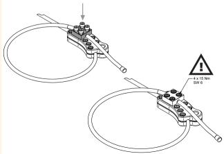
Connect the end lock to the IND-EB-40 with bolt and peg.
