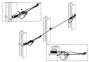
Add 300 kg pretension to the cable system. [134 mm = 300 kg]
